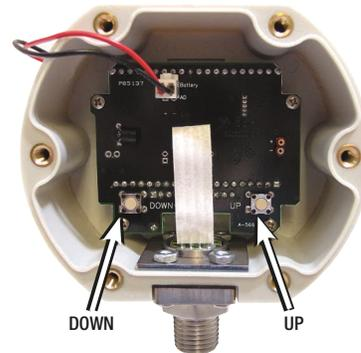
With the gauge off, press and hold the DOWN calibration button, and also press the front button.
