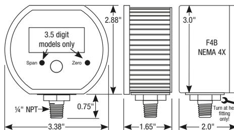
3.5 digit models use plastic caps on potentiometers, F4 covers are nylon screws with o-rings. 4 digit models use internal buttons.
